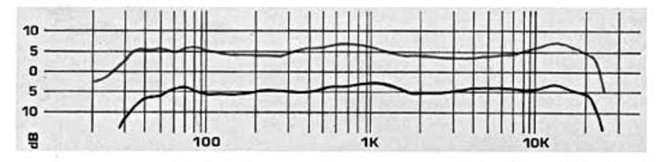
On-axis response in controlled reverberant field environment. Curves are offset 10 dB for clarity of presentation.
